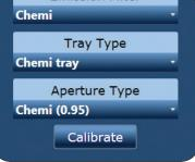
Focus is affected by the choice of emission filter, aperture setting and tray position. There are many possible combinations of these three settings (~48) so a calibration method for all of these combinations is provided in the SETTINGS tab.
