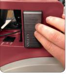
3. Disconnect the camera USB from the right angle adapter.
