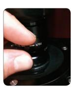
6. Adjust focus until image is clearly focused then turn focus ring until the image is slightly out of focus in the "NEAR" direction.
