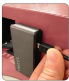
6. Connect the Hub USB mini cable to the right angle adapter.
