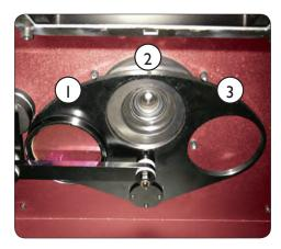
Remove the lens from the packaging and insert it into the open filter position. The filter ring is threaded. Turn the filter clockwise to tighten. Take care not to cross the threads.
