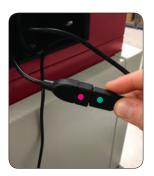
4. Slide the camera USB cable through the cable guide and plug it into the Hub.
