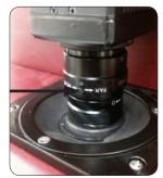
8. Lock focus ring in place with focus ring locking screw.
