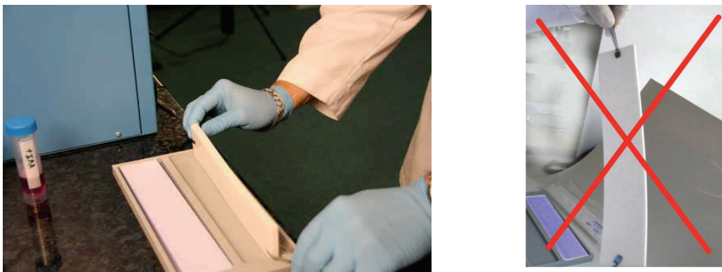
Fig. 6: Removal of excess buffer from the wicks. Always hold the wicks horizontally.
