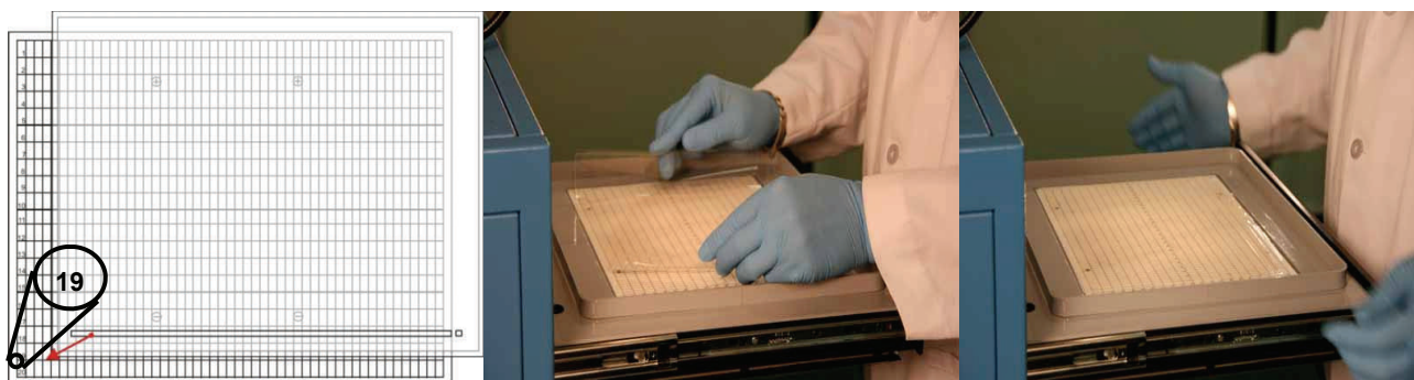
Fig. 5: Placing Flatbed Large gel on the cooling plate.
