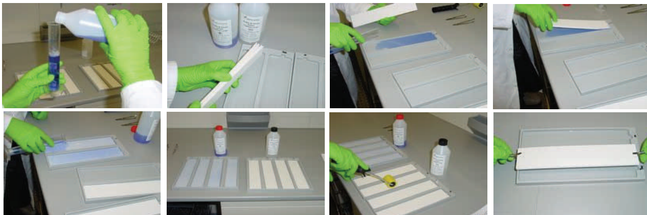
Fig. 1: Soaking stacks of four paper wicks in 80 mL electrode buffer. First pour 40 mL buffer into the empty PaperPool compartment, then lay the stack of paper wicks into the PaperPool and add another 40 mL buffer.
