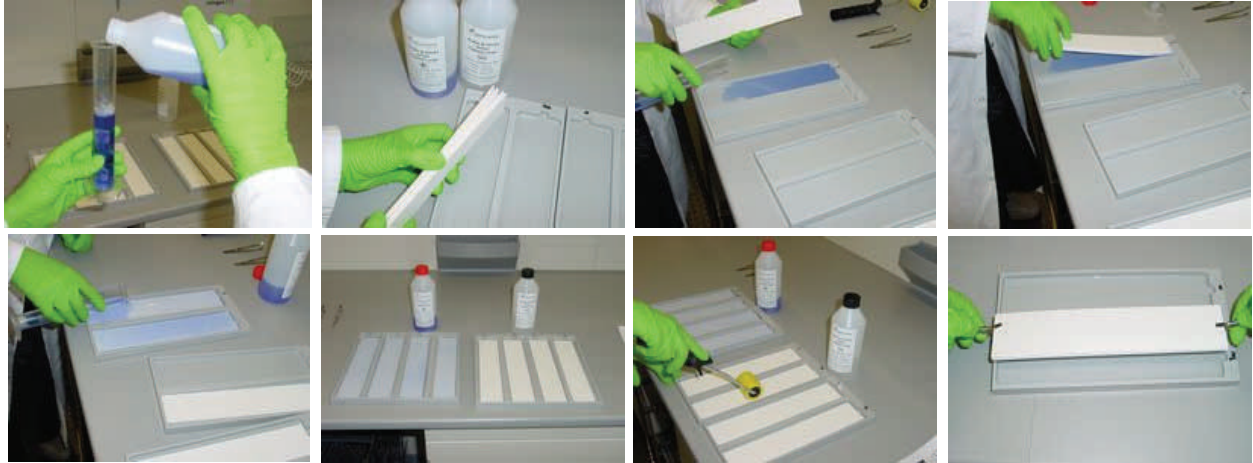
Fig. 5.1: Soaking stacks of four paper wicks in 80 mL electrode buffer. First pour 40 mL buffer into the empty PaperPool compartment, then lay the stack of paper wicks into the PaperPool and add another 40 mL buffer.
