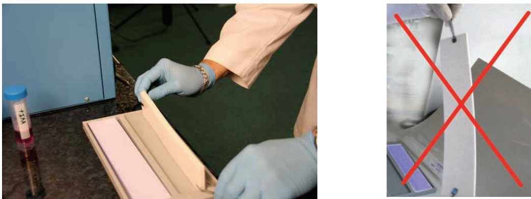
Fig. 5.6: Removal of excess buffer from the wicks. Always hold the wicks horizontally.
