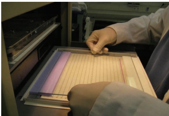
Fig. 5.9: Placing a glass plate on the buffer wicks for optimal contact of wicks and gel and to ensure a straight front.
