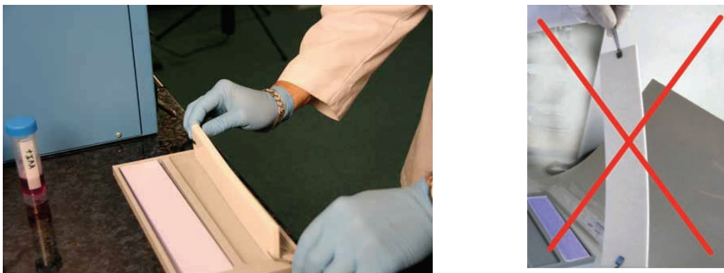
Fig. 5.6: Removal of excess buffer from the wicks. Always hold the wicks horizontally.
