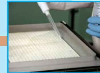
Application of a few mL cooling contact fluid
