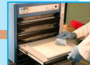
Clean the cooling plate by simply wiping off the cooling fluid and remains of the buffers
