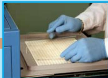
Placing the gel on the cooling plate
