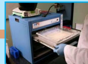
After electrophoresis remove the gel for direct scanning (DIGE) or post-staining
