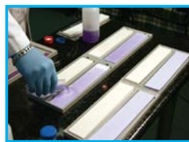
Soaking the filter paper wicks with electrode buffer. The anodal solution is color coded blue
