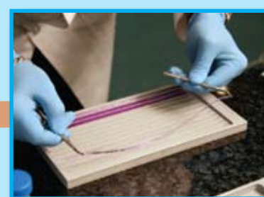
Equilibration of the IPG strips with the provided equilibration buffer, only urea, DTT, and iodoacetamide need to be added.
