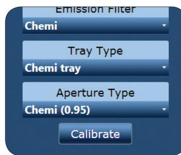
Focus is affected by the choice of emission filter, aperture setting and tray position. There are many possible combinations of these three settings (~48) so a calibration method for all of these combinations is provided in the SETTINGS tab.
