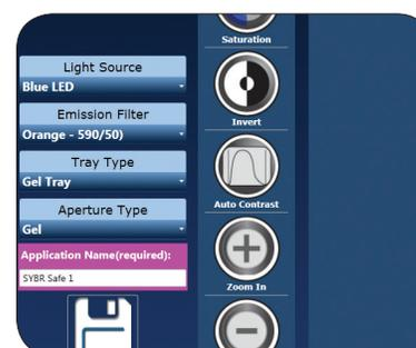
The Custom Application option builds the application based on the original applications parameters, which have defined sensitivity levels, darkmaster correction, and auto-exposure methods.
